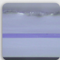
150x transverse view of the implant shell including the visual barrier-layer indicator BluSeal®
